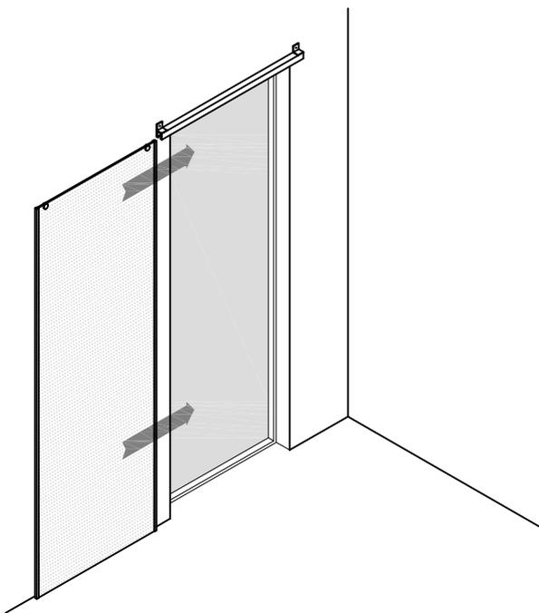
**7** From the side, slide the DecoGlide™ onto the track
