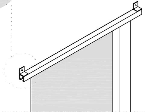
**6** Fix angles and attached track to wall using your selected fixings
