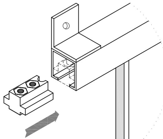
**8** Place end stops onto track ends and screw them firmly into track using screws provided
